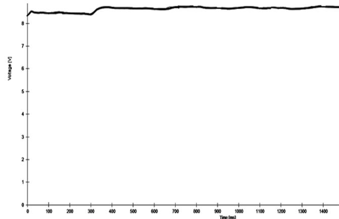
Figure 14: Graph of  $V_{DC}$  when  $V_{AC}$  is 7.23V and dynamo frequency is 530.52Hz
