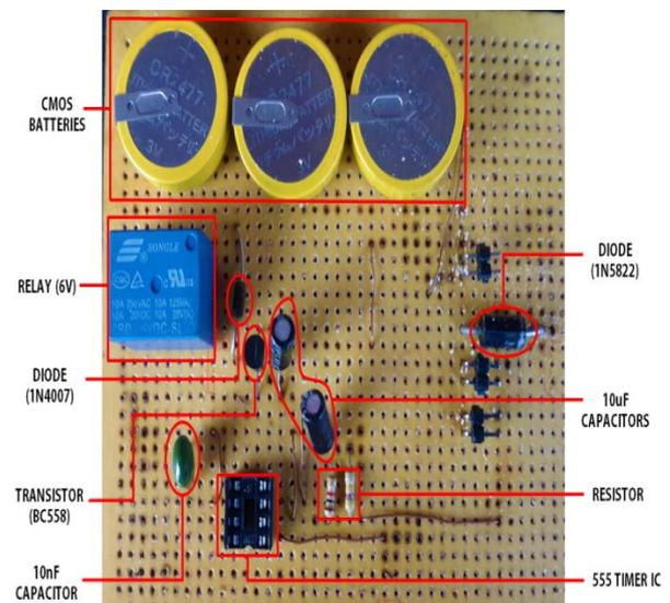
Figure 8: Switching mechanism circuit implementation
