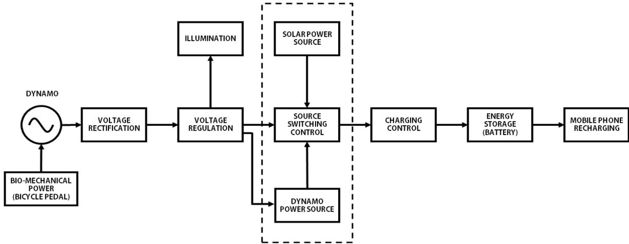
Figure 1: Solar-Dynamo Mobile Phone Charger
