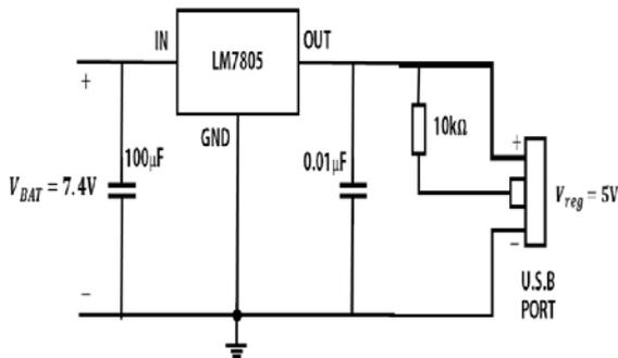
Figure 4: Mobile Phone Recharging Circuit
