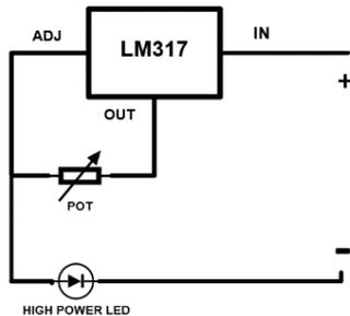
Figure 6: Illumination Circuit
