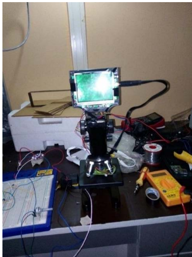
Figure 4: Attaching the TFT LCD display on the microscope
