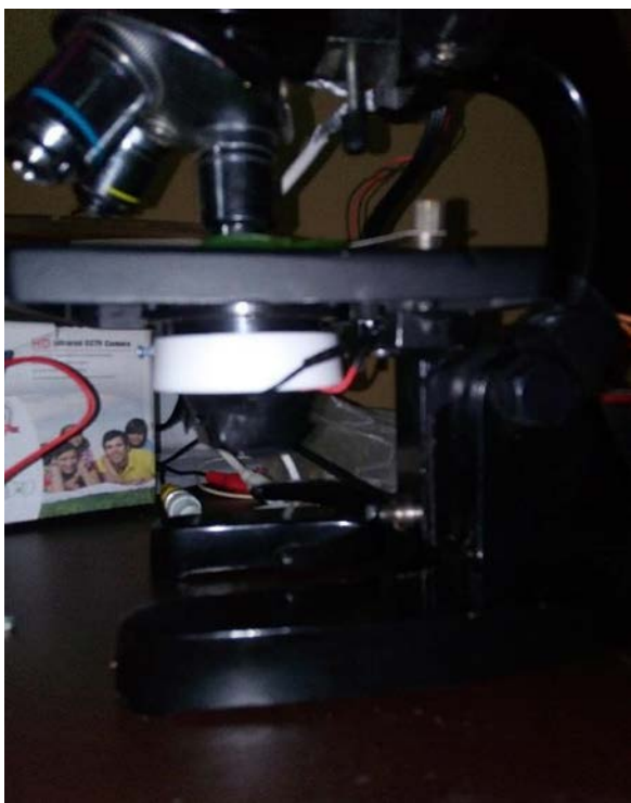
Figure 3: Attachment of the light control system to the microscope
