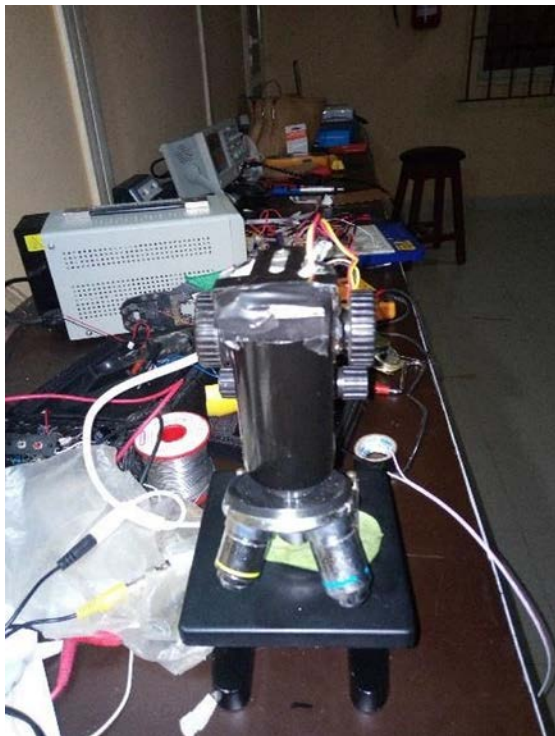
Figure 2: Insertion of the camera lens and the image sensor inside the microscope
