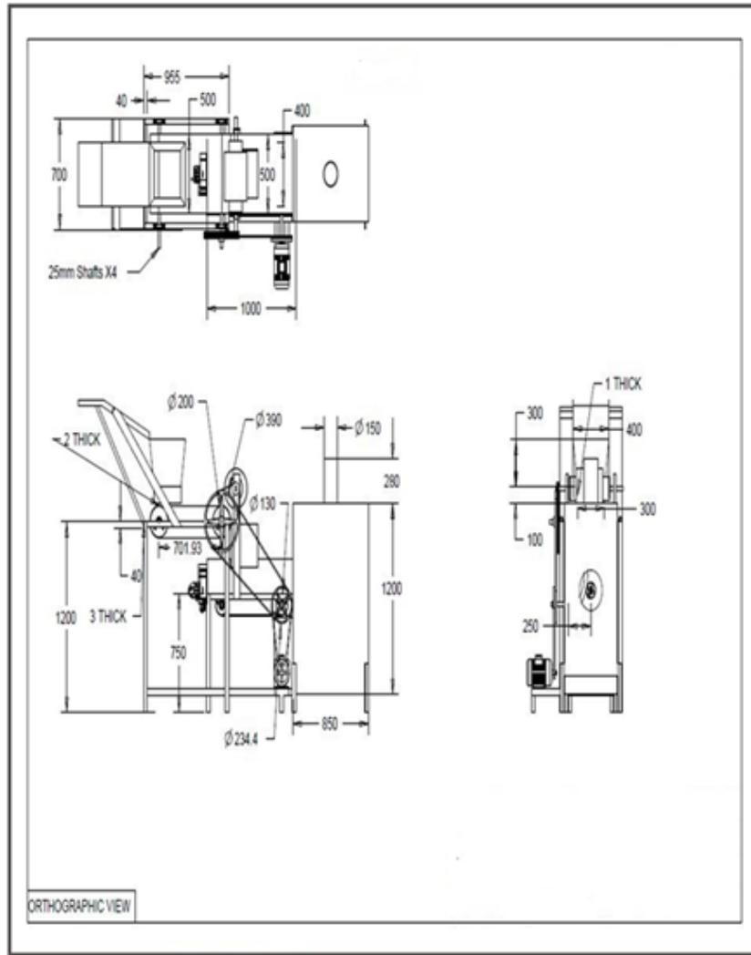
Figure 3. The orthographic drawings of the solid waste sorting machine
