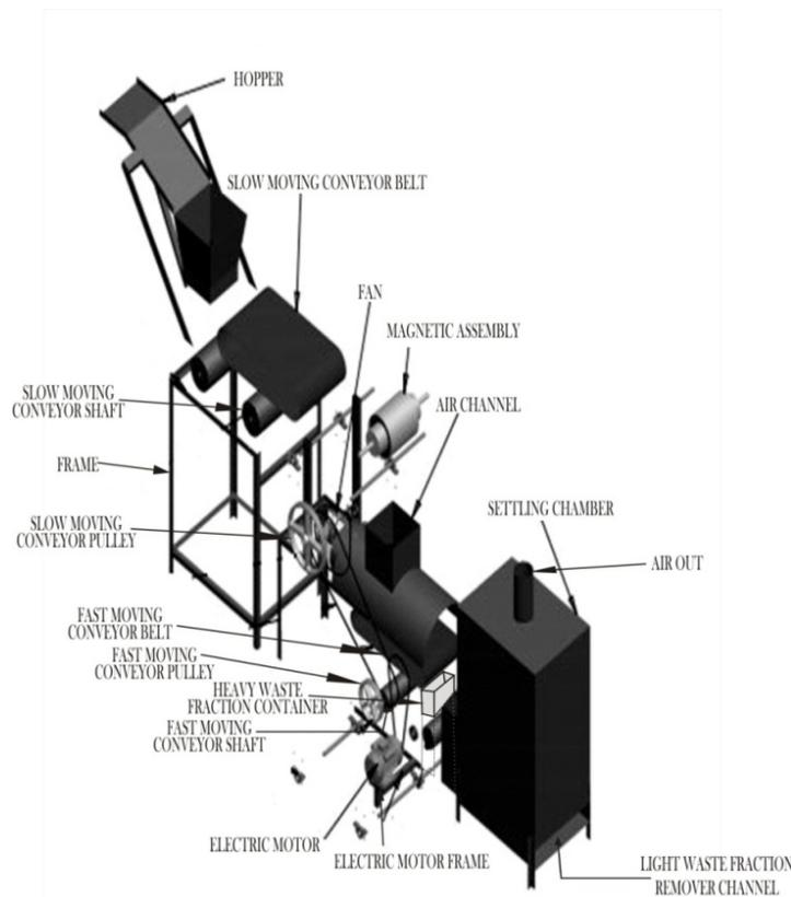
Figure 2. An exploded view of the fabricated solid waste sorting machine
