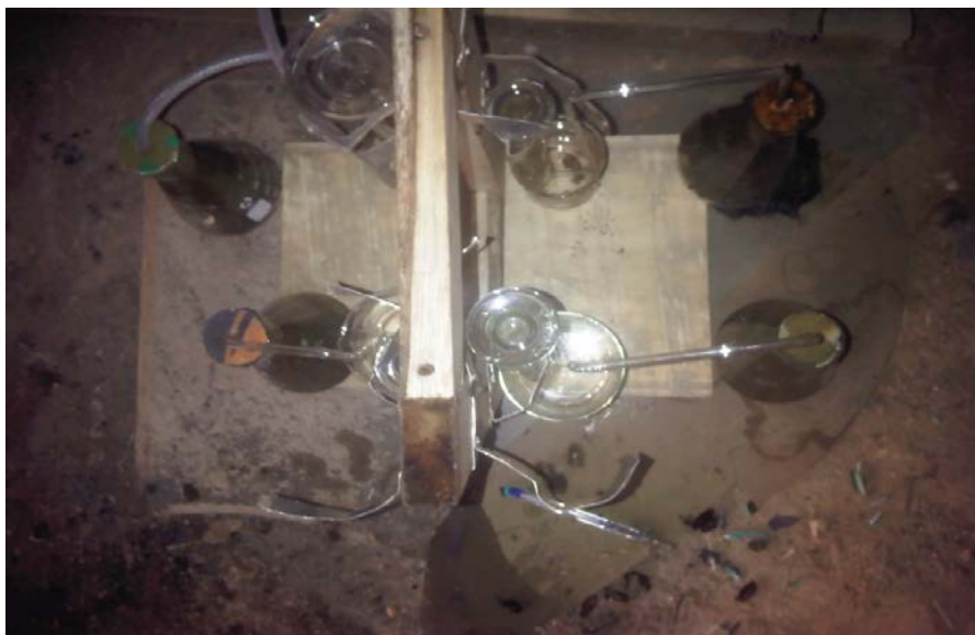
Figure 1: Experimental set up of anaerobic digester with substrates
