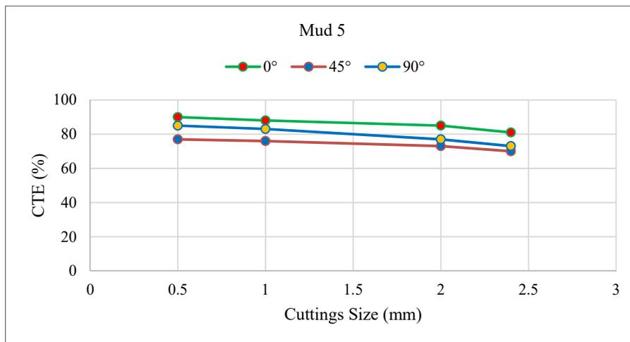
**Figure 7:** Effect of different cuttings sizes on CTE using Mud 5 (Mud 1+ 10 g of Henna + 10 g of Lignite).
