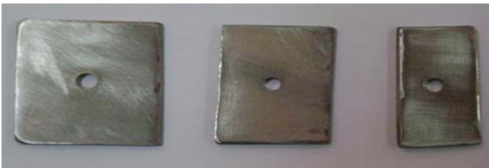
Figure 1: Cut and Polished corrosion test coupons of varied dimension
