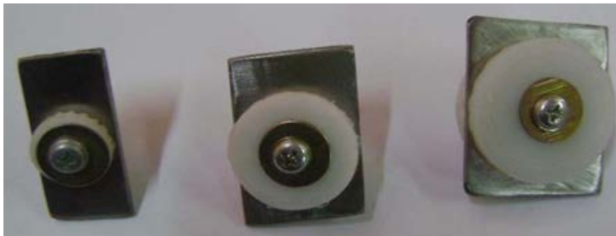
Figure 3: Multiple Crevice Assembly for Crevice Corrosion Test according to ASTM G78. Coupon Analyses
