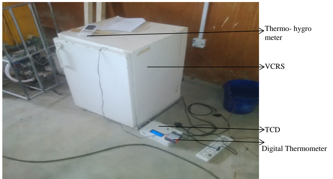
Figure 4. Developed MCBRCS Tested on No - Load Condition
