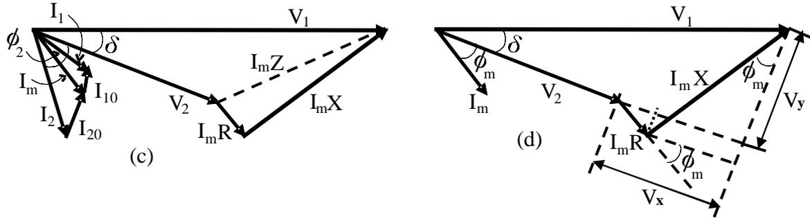
Fig. 2: (a) One-Line Diagram of the MTL; (b) Nominal-Π Equivalent Circuit of the MTL; (c) Phasor Diagram relative to the Equivalent Circuit; (d) Short-Line Equivalent of the Nominal-Π Equivalent Circuit Phasor Diagram
