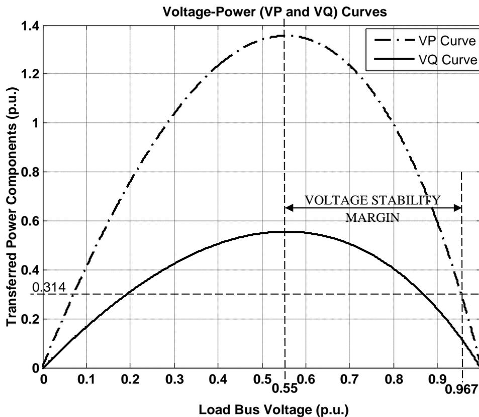
Fig. 3: VP and VQ Curves for PML and Maximum MVar Determination (being a MATLAB Plot from the Relevant Load Flow Equations)
