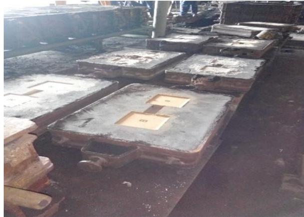
Figure 4: Cast TWDI samples in binder/ sand formulations
