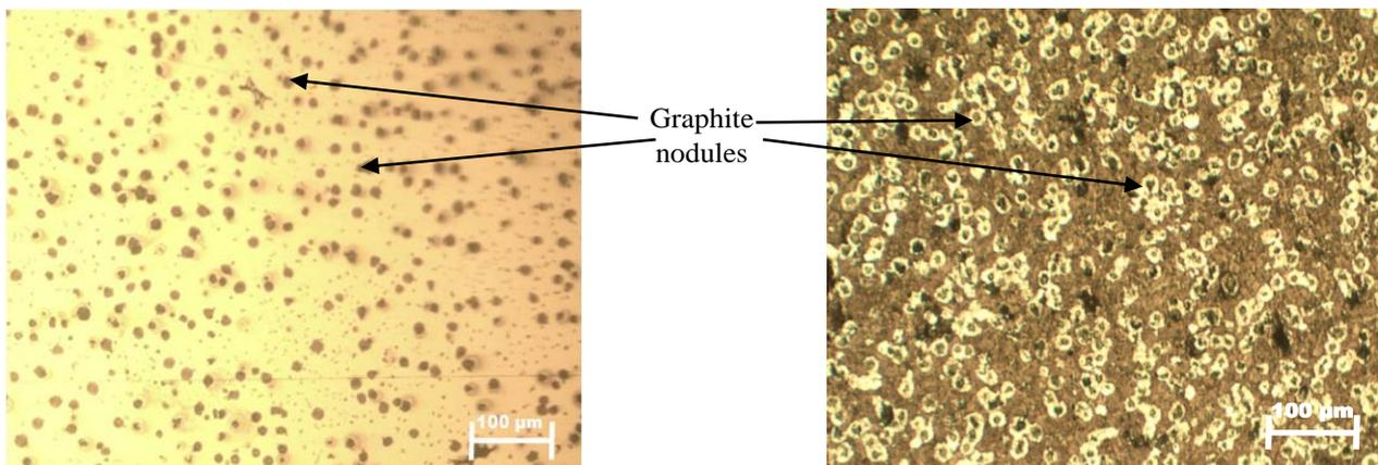
Figure 11: Micrographs of TWDI cast in Sugar syrup bonded sand (a) Unetched (b) Etched
