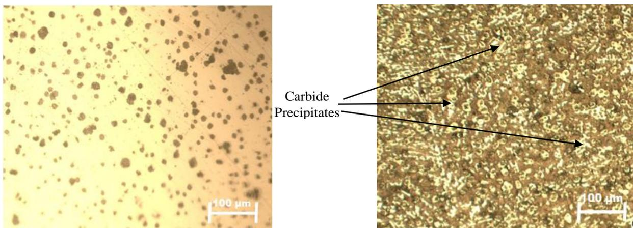
Figure 12: Micrographs of TWDI cast in Corn Starch bonded sand (a) Unetched (b) Etched
