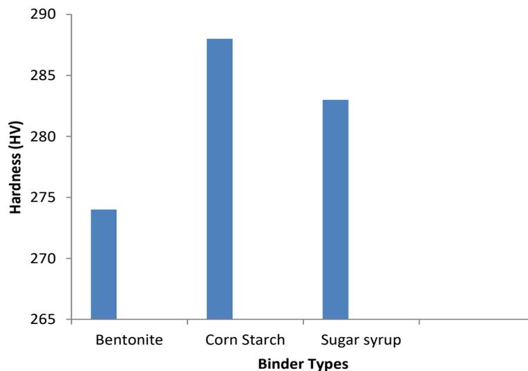
Figure 9: Hardness of cast TWDI samples with Binder Types
