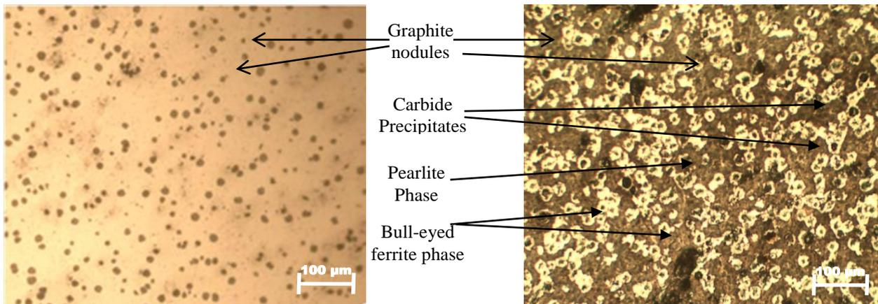
Figure 10: Micrographs of TWDI cast in Bentonite bonded sand (a) Unetched (b) Etched
