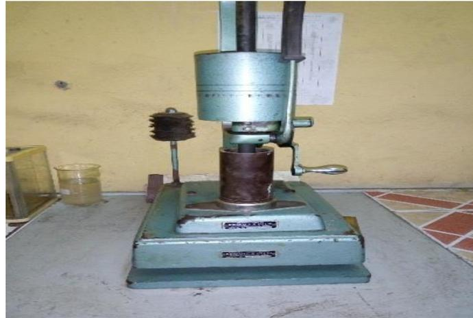
Figure 2: Ramming of Sand/Binder Formulations using Ridsdale Rammer
