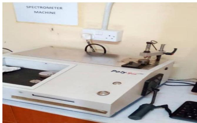
Figure 5: Spectrometer for chemical composition analysis (Machine Tools Ltd, Osogbo)
