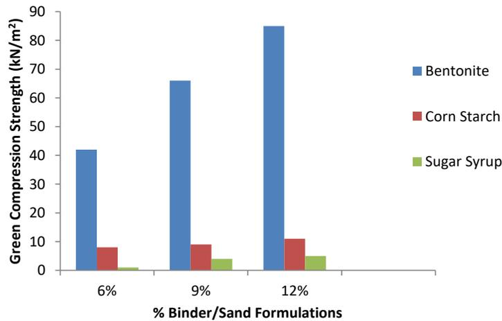
Figure 6: Chart of Green Compression Strength with % binder/Sand Formulations
