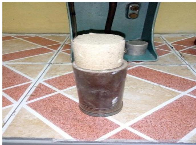
Figure 1: Test piece for mould property analysis
