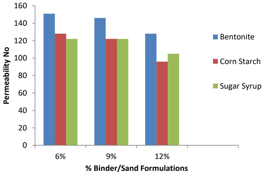
Figure 8: Chart of Permeability (No) with % binder/Sand Formulations
