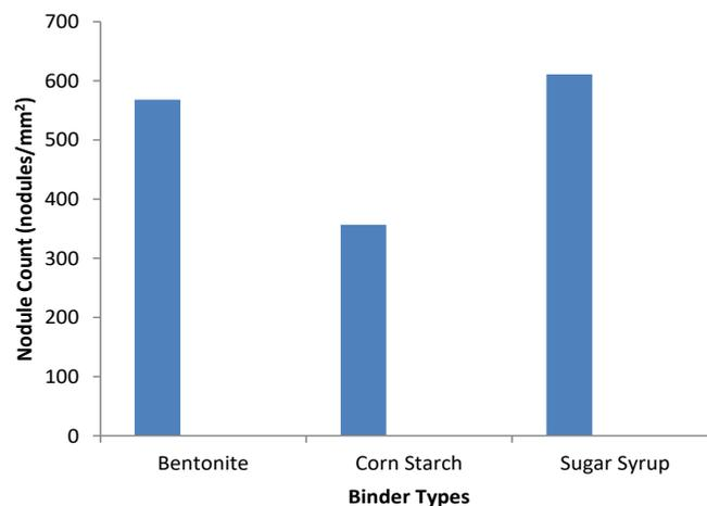
Figure 14: Nodule count/mm<sup>2</sup> of cast TWDI samples with Binder Types
