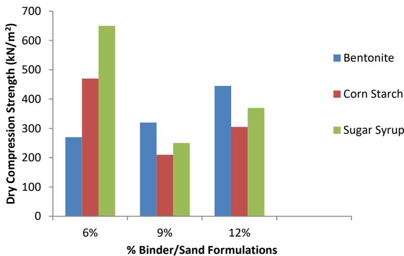
Figure 7: Chart of Dry Compression Strength with % binder/Sand Formulations
