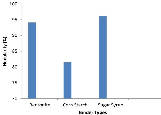
Figure 13: Nodularity (%) of cast TWDI samples with Binder Types
