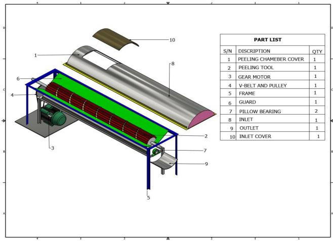
Figure 1: Exploded View of Automated Cassava Peeler
