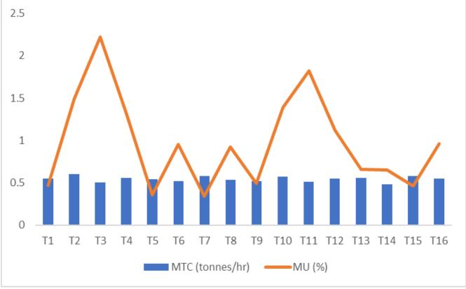
Figure 12: Effect of Different Treatments on the Performance Evaluation of the Cassava Peeler.
