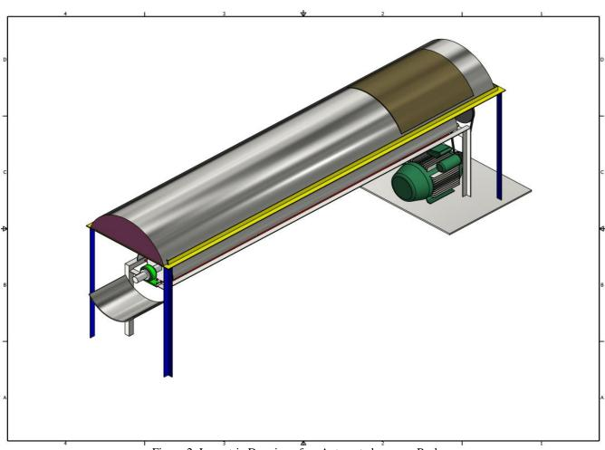
Figure 2: Isometric Drawing of an Automated cassava Peeler
