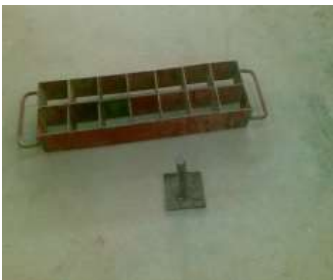
Figure 3(a): (76.2 mm cubic mould and ram)
