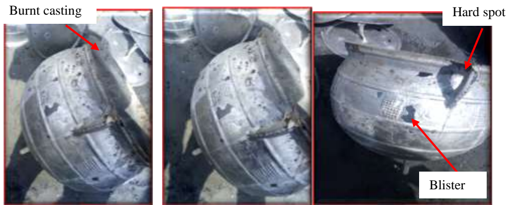
Plate II: Burnt castings with hard spots, and blisters
