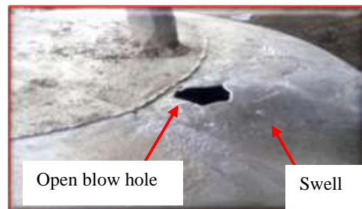
Plate IIc: Casting with blow holes and swell
