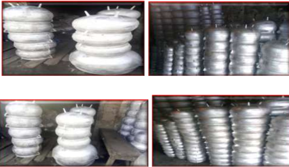
Plate I Piles of some of the observed defect-free pot castings from the foundry shops at PantekaTudunwada
