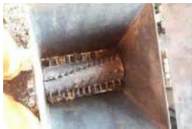
Figure 10 (a): Image of modified cutter. Figure 10 (b): Drawing of modified cutter.
