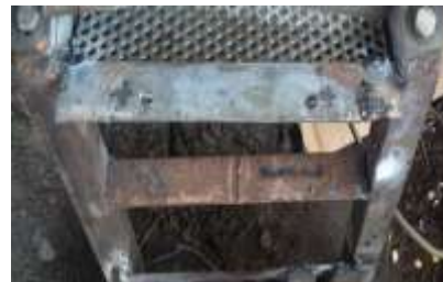
Figure 6(b): Mesh welded to frame.
