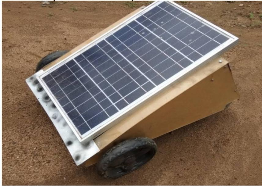
Fig 6: Aerial view of the constructed Automated Lawn Mower
