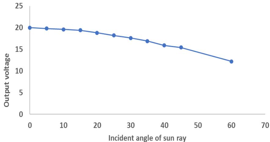
Figure 9: Relationship between the Output Voltage of Battery and Angle of Incidence of the Sun rays
