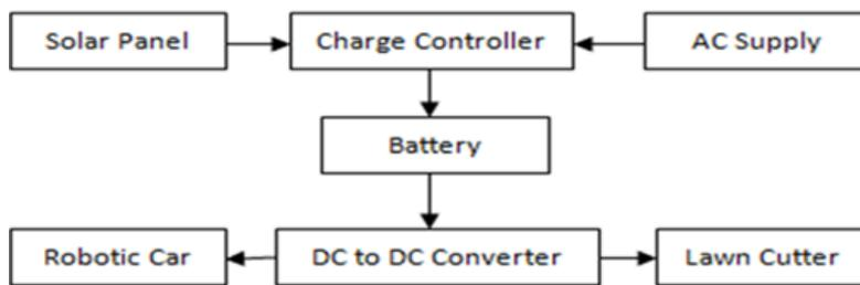
Fig 1: System's Block diagram
