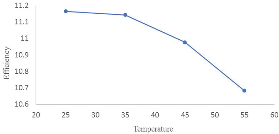
Fig 8: Relationship between the Efficiency of solar cell and Temperature.
