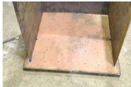
Figure 2b: Fabricated Steam Box
