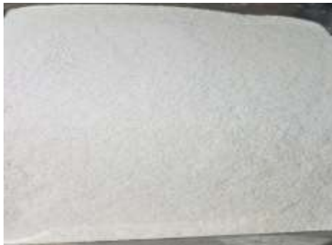
Figure 2: Calcium carbide residue used as the reinforcement in the composite
