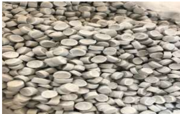
Figure 1: Polypropylene pellets used as Matrix material for the composite
