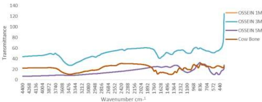
Figure 13: FTIR Spectra for Ossein samples
