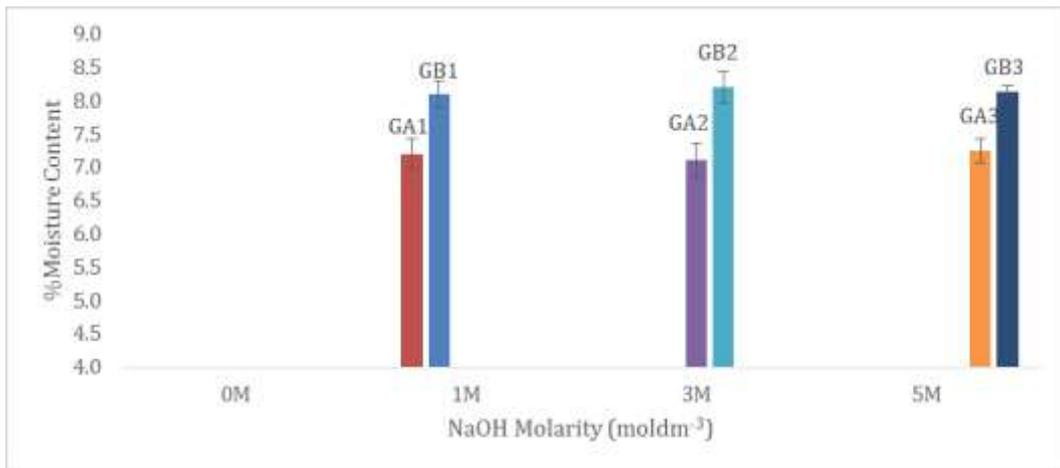
Figure 9: Chart of % moisture content versus NaOH molarity
