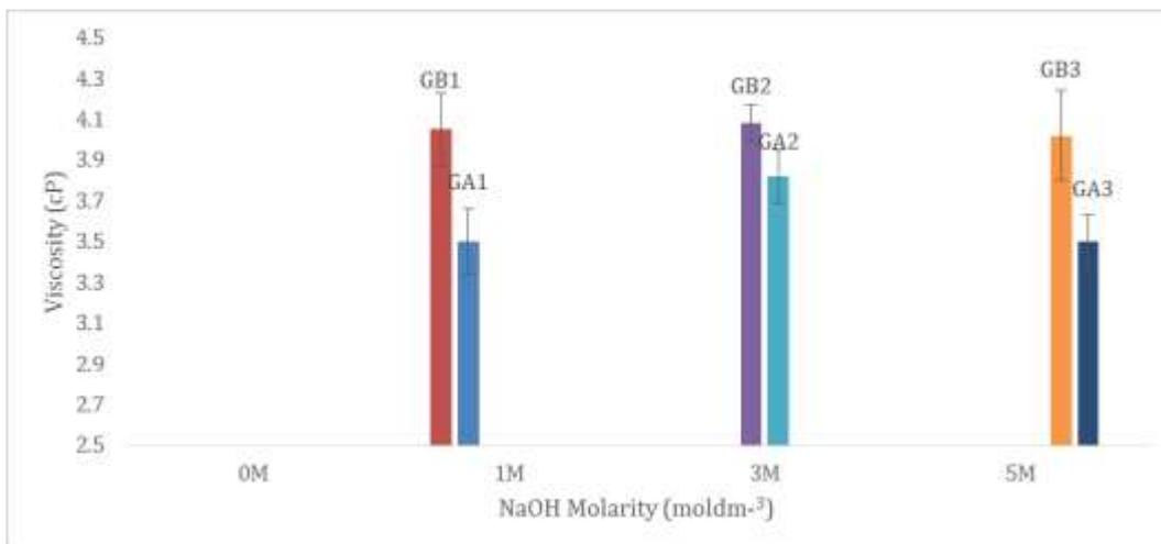
Figure 7: Chart of viscosity versus NaOH molarity of extracted gelatin
