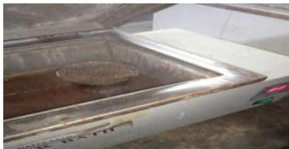
Figure 3: Extraction process for samples in the water bath.
