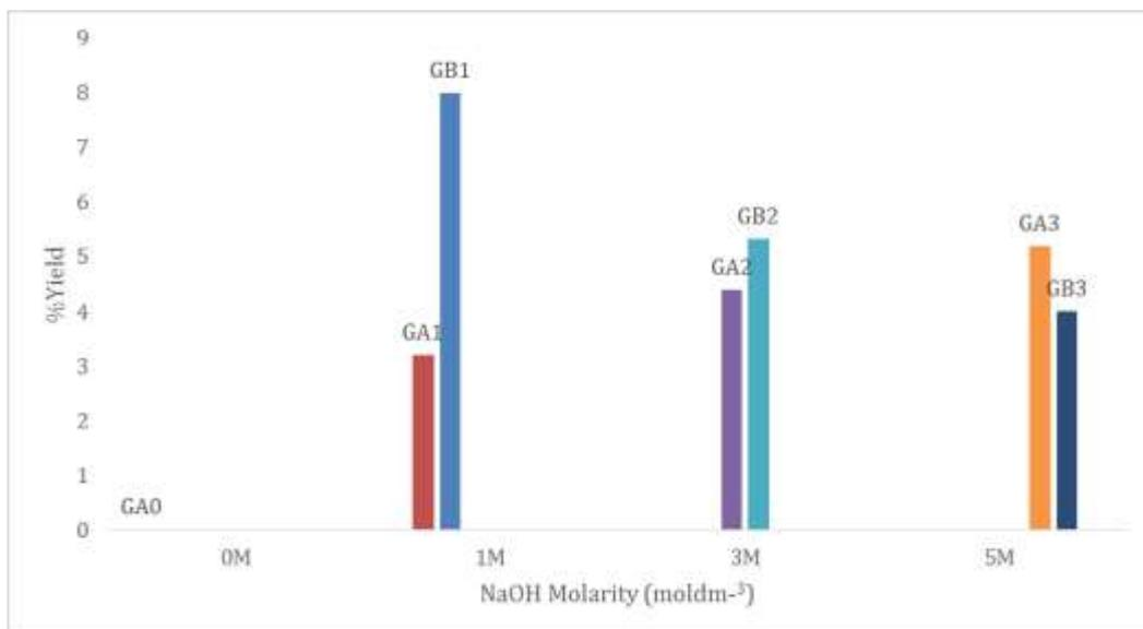
Figure 6: Chart of yield versus NaOH molarity for size reduced and original sample
