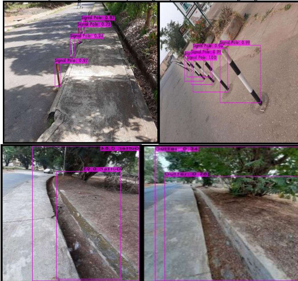
Figure 4: Gutter and Bollards Prediction Outputs
