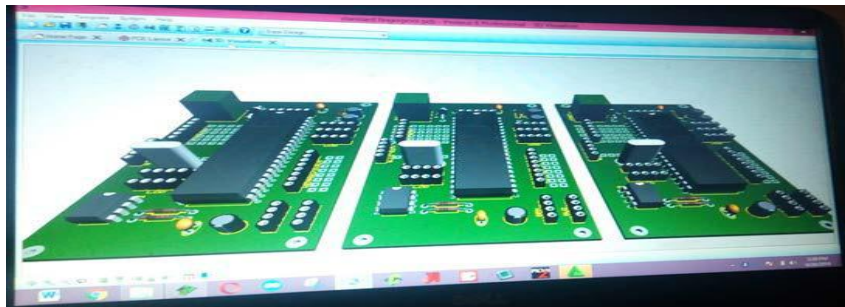
Figure 6: PCB design on proteus.
