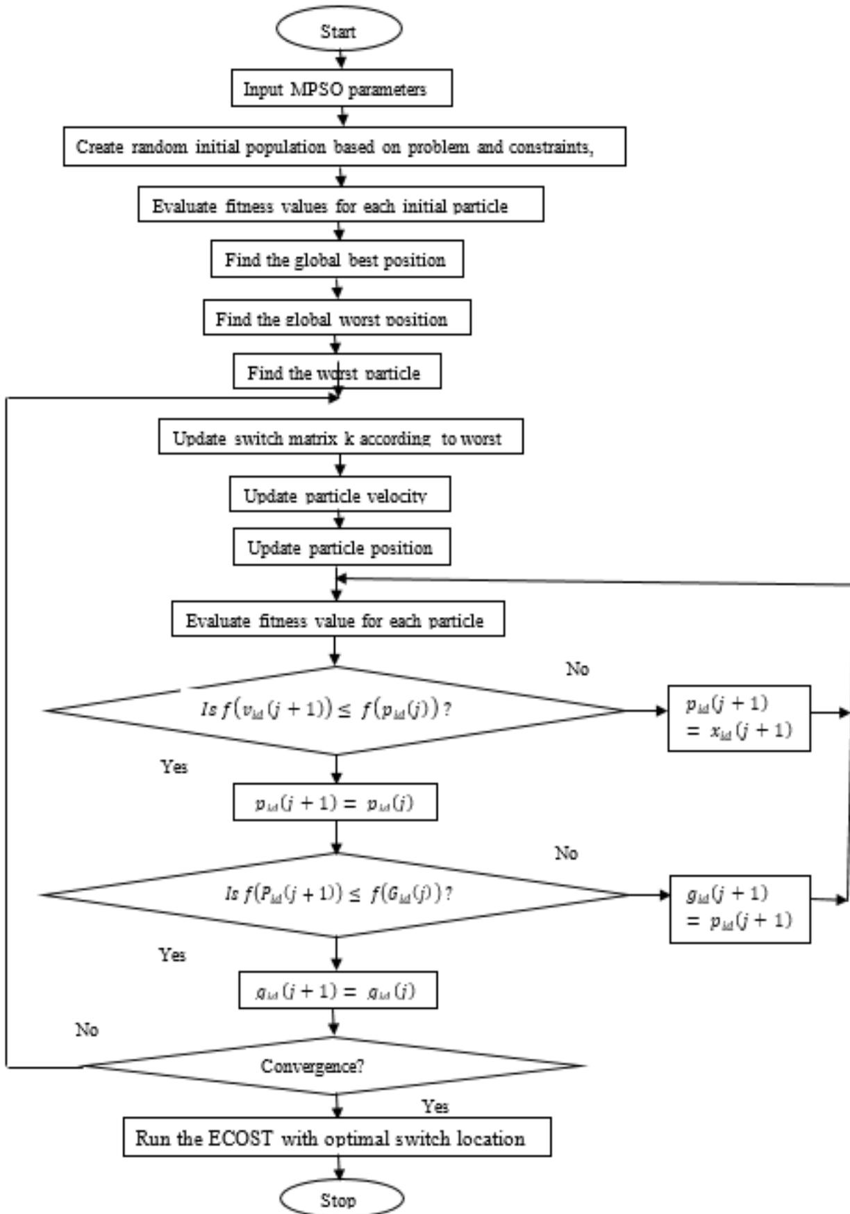
Figure 2: Flow chart for optimal placement of switches using MPSO
