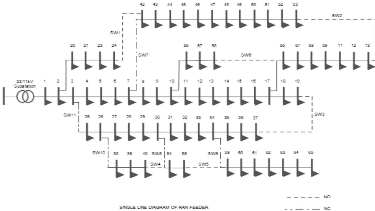
Figure 1: Single line diagram of the 11 kV Ran feeder of JEDC Distribution Company of Bauchi
