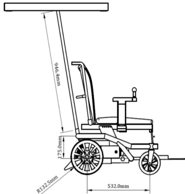
Figure 3: Side view of the design
