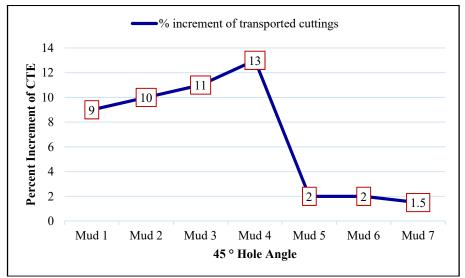
Figure 10: Percent increment of transported cuttings for different mud systems at 45° hole-angle.
