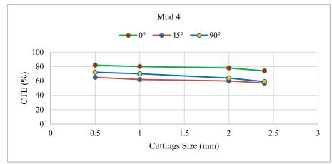
Figure 6: Effect of different cuttings sizes on CTE using Mud 4 (Mud 1+ 10 g of Henna + 8 g of Lignite).
