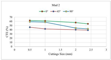
Figure 4: Effect of different cuttings sizes on CTE using Mud 2 (Mud 1 +10 g of Henna).
