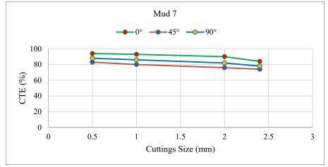
Figure 9: Effect of different cuttings sizes on CTE using Mud 7 (Mud 1+ 10 g of Henna + 15 g of Lignite).
