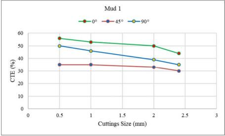
Figure 3: Effect of different cuttings sizes on CTE using Mud 1 (Base mud).
