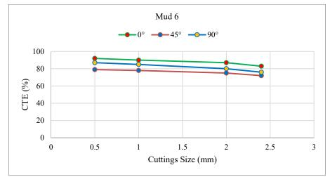
Figure 8: Effect of different cuttings sizes on CTE using Mud 6 (Mud 1+ 10 g of Henna + 12 g of Lignite).
