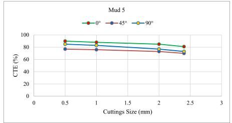
Figure 7: Effect of different cuttings sizes on CTE using Mud 5 (Mud 1+ 10 g of Henna + 10 g of Lignite).
