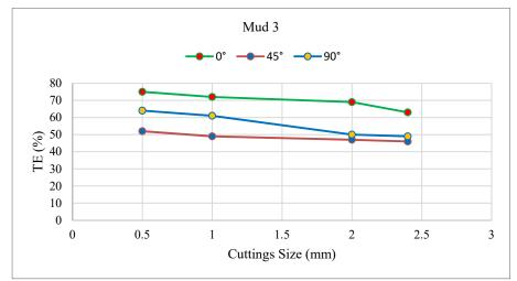
Figure 5: Effect of different cuttings sizes on CTE using Mud 3 (Mud 1+ 10 g of Henna + 5 g of Lignite).
