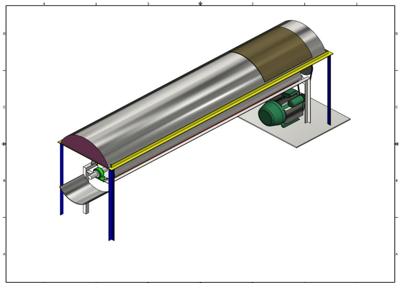
Figure 2: Isometric Drawing of an Automated cassava Peeler
