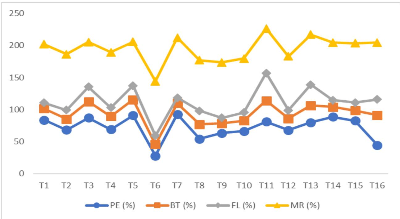
Figure 11: Effect of Different Treatments on the Performance Evaluation of the Cassava Peeling Machine
