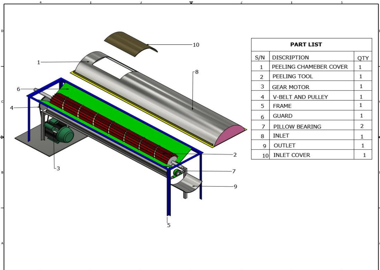
Figure 1: Exploded View of Automated Cassava Peeler
