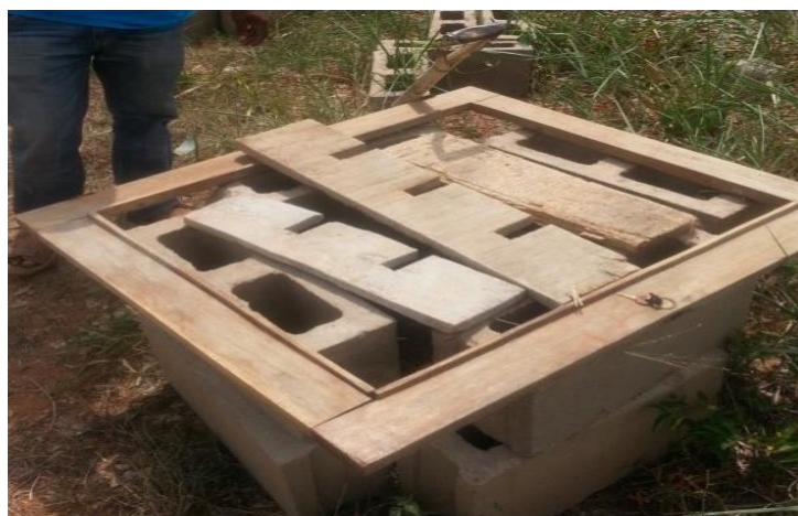
Figure 2: Produced termite resistant sandcrete blocks on earthen surface.
