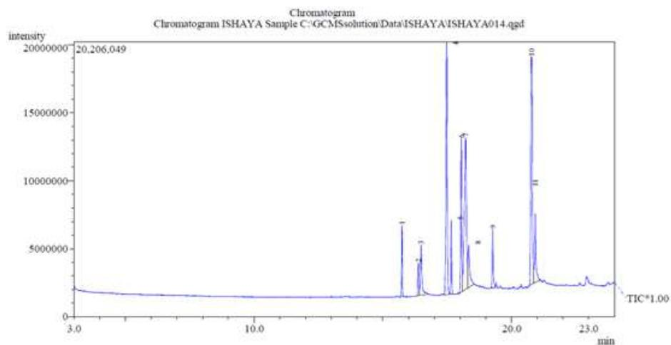
Figure 4: Chromatograph of biodiesel sample-AM.1:12 - mass spectral showing the scan peaks
