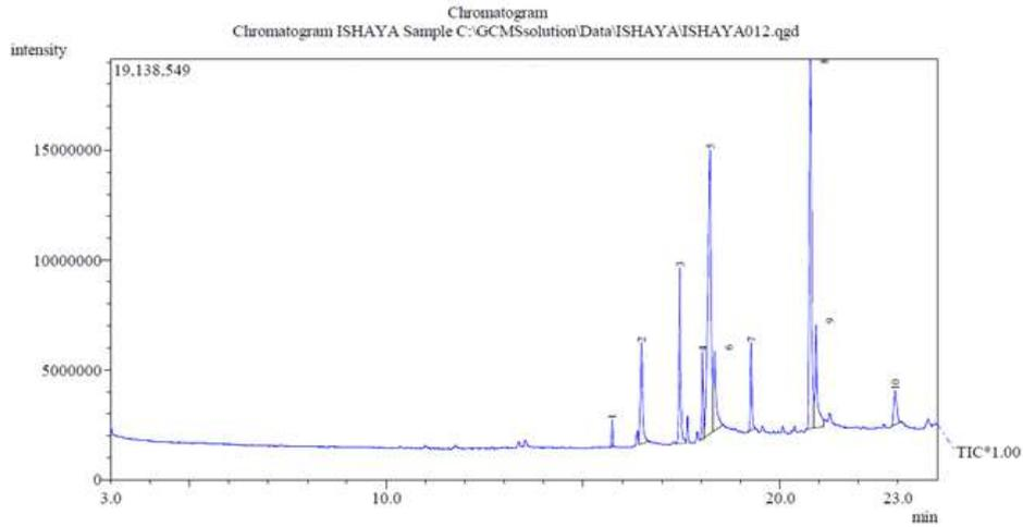
Figure 3: Chromatograph of biodiesel sample-AM.1:9 - mass spectral showing the scan peaks
