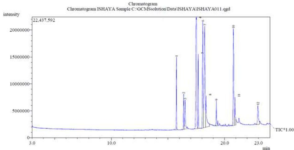
Figure 2: Chromatograph of biodiesel sample-AM.1:6 - mass spectral showing the scan peaks
