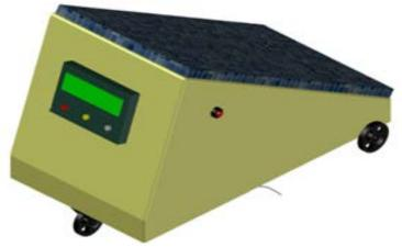
Fig 5: The 3-D design of the Automated Lawn Mower
