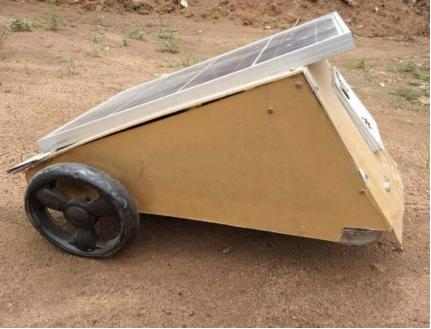
Fig 7: Side view of the constructed Automated Lawn Mower.
