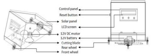
Fig 3: Isometric and front view of the automated lawn cutter
