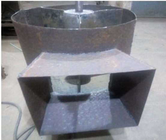
Figure 2: Mixing Drum with the hopper
