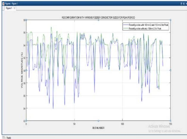
Figure 10: Voltage Profile of the Proposed Configuration with 100mm<sup>2</sup>&150mm<sup>2</sup> and with only 150mm<sup>2</sup> Feeder Conductor Sizes for Peak Period
