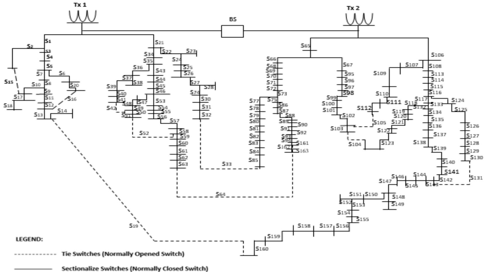
Figure 3: The Existing Configuration of the Ugbowo 2 x 15 MVA, 33/11 kV Distribution Network
