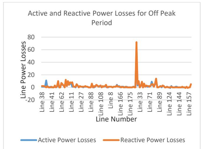
Figure 13: Active and Reactive Line Losses for Base Configuration of each Connected Bus for Off Peak Period.
