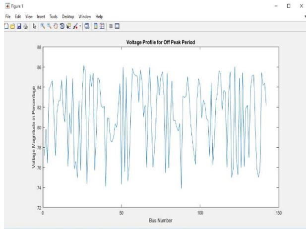
Figure 6: Voltage Profile of Existing or Base Configuration for Off Peak Period with 100mm<sup>2</sup> and 150mm<sup>2</sup> Conductor Sizes
