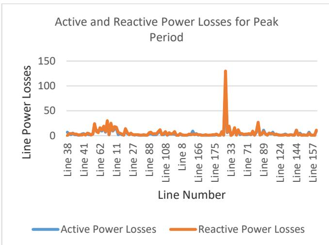
Figure 12: Active and Reactive Line Losses for Base Configuration of each Connected Bus for Peak Period.
