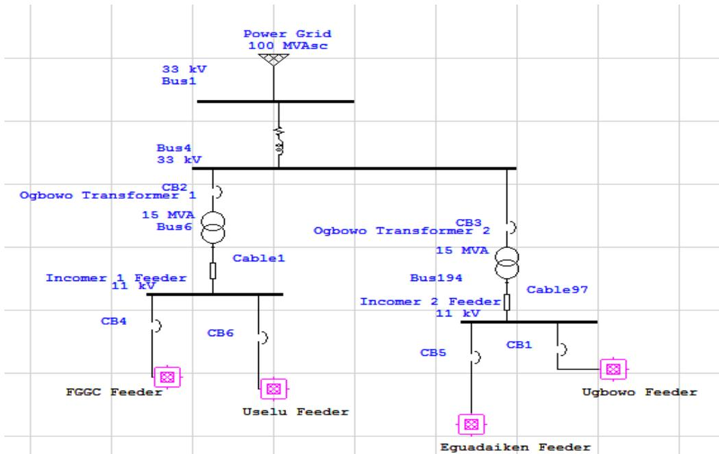
Figure 4: Single Line Diagram of Ugbowo 2 x 15 MVA, 33/11 kV Distribution Network in ETAP Environment
