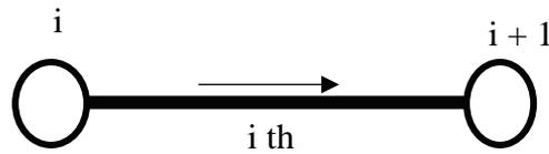
Figure 1: Schematic Representation of a Feeder Line Connecting Two Adjoining Buses
