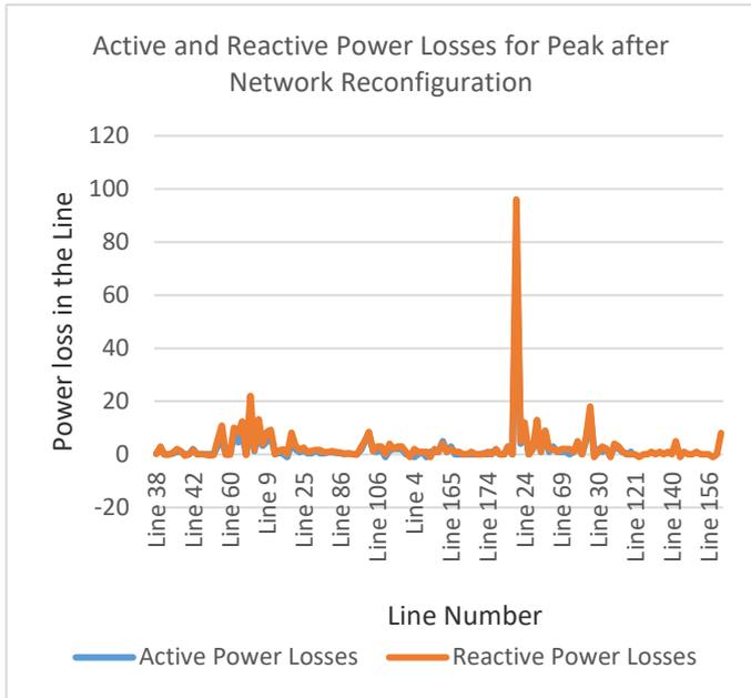
Figure 14: Active and Reactive Line Losses for each Connected Bus for Peak Period after Optimal Network Reconfiguration.
