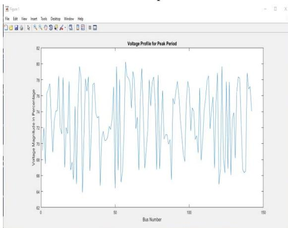
Figure 5: Voltage Profile of Existing or Base Configuration for Peak Period with 100mm<sup>2</sup> and 150mm<sup>2</sup> Conductor Sizes
