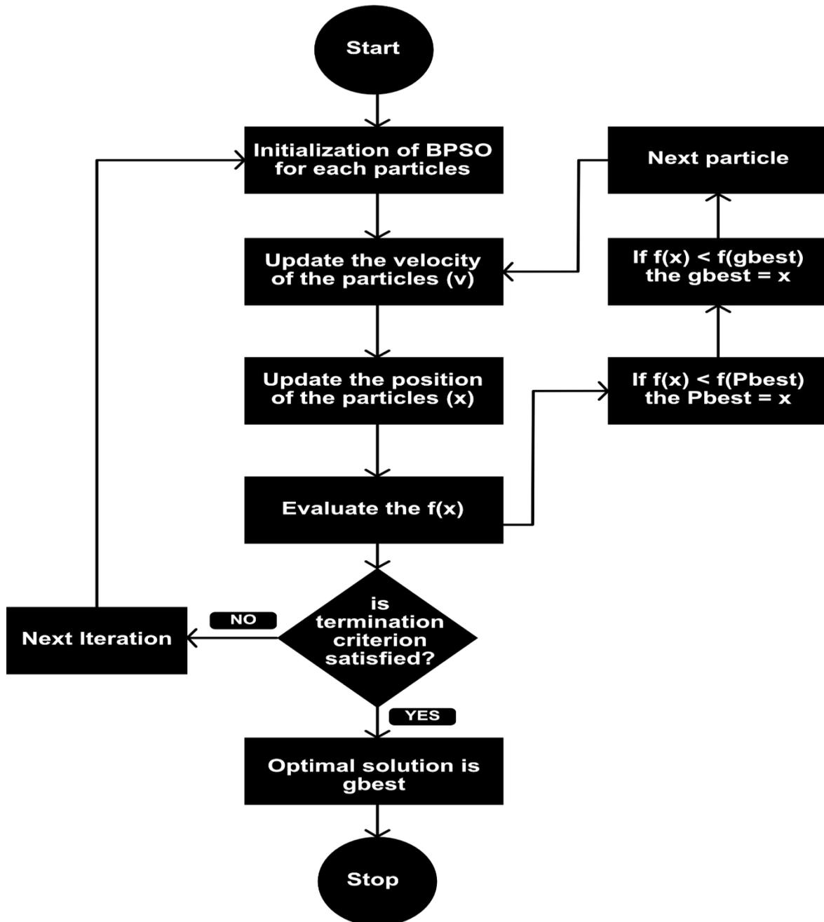
Figure 2: The Flow Chart of BPSO for Optimal Network Reconfiguration of Distribution System
