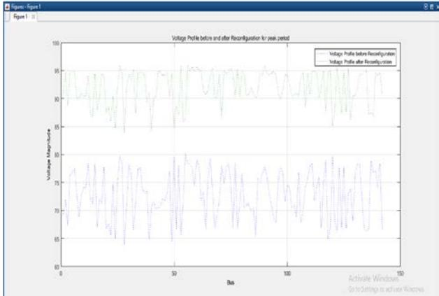
Figure 8: Voltage Profile of the Existing and the Proposed Configuration with 100mm<sup>2</sup> and 150mm<sup>2</sup> Feeder Conductor Sizes for Peak Period
