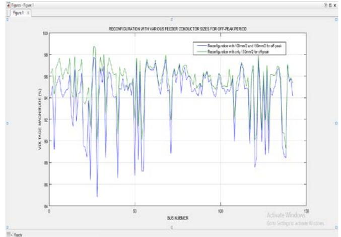
Figure 11: Voltage Profile of the Proposed Configuration with 100mm<sup>2</sup>&150mm<sup>2</sup> and with only 150mm<sup>2</sup> Feeder Conductor Sizes for Off Peak Period
